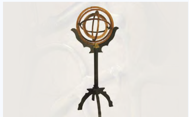
Fig. 3. Spherical astrolabe: the most sophisticated ancient astronomic instrument used to determine ecliptic or equatorial coordinates of celestial bodies
