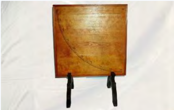
Fig. 1. Solar Quadrant: used for measuring the level of the Sun and the inclination of the ecliptic – Earth's orbit – to the celestial equator.
