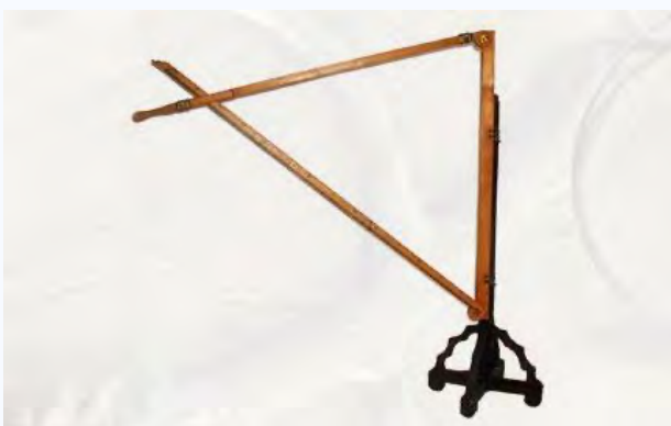
Fig. 2. Parallactic ruler or Triquetrum: An instrument used to measure the altitude of Sun (the apparent change in its position resulting from the movement of the observer staying on Earth)
